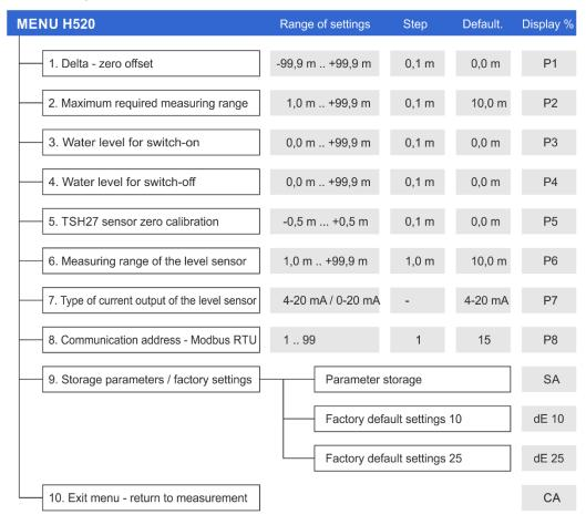
Entering the menu, changing individual parameters, saving them to the unit's memory and exiting the menu is done using 3 control buttons. The buttons are accessible from the rear of the display panel.
