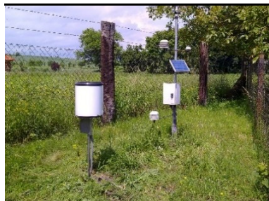
Small weather station
