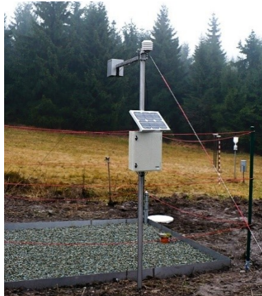
Snow gauge station complete Snow gauge station
